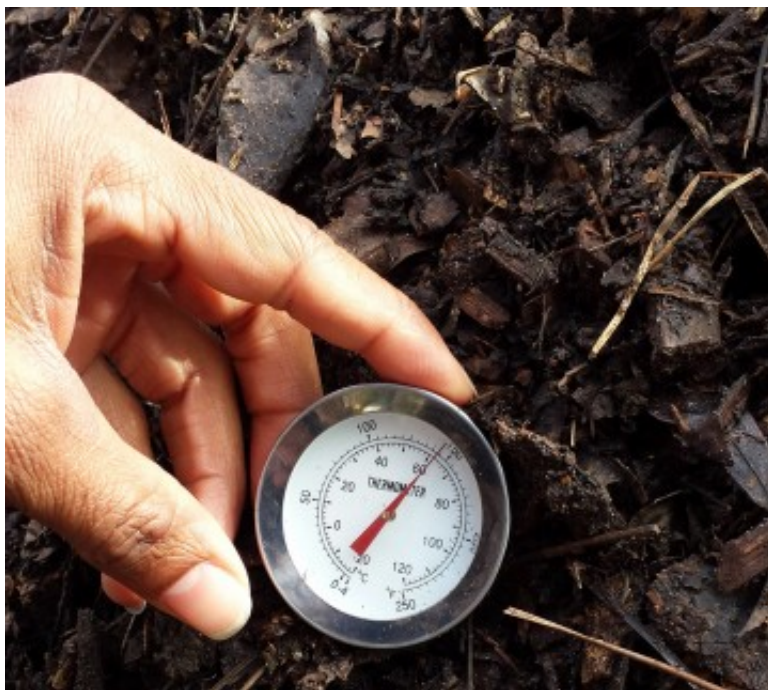
Sundiata Ameh-El uses a compost thermometer, designed like a meat thermometer but with a longer stem, to monitor temperatures of the active compost heaps at Compost Community.
